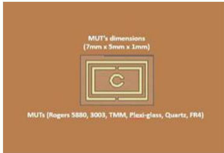
Fig. 7 Dimension and position of the MUTs in the ground plane of the proposed sensor
